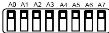
Figure 6: MAC address DIP switches
